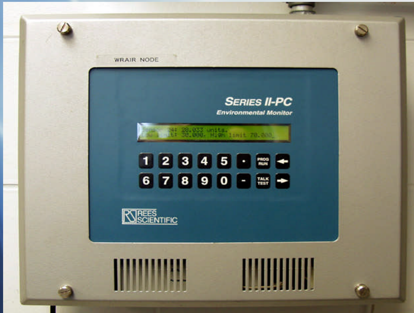
Computerized room temperature & humidity monitoring system
